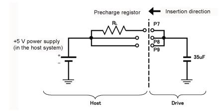
It is necessary to choose pre-charge resistor  $R_L$  value, which is in permissible range of +5V power supply specification at the host system.
